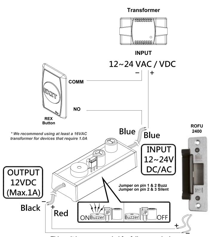
This unit is recommended for fail secure devices
