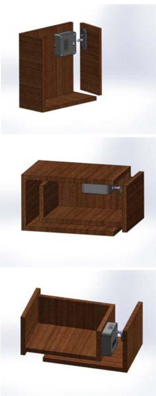
Swing Door Application (Pivoting Door Mount)
