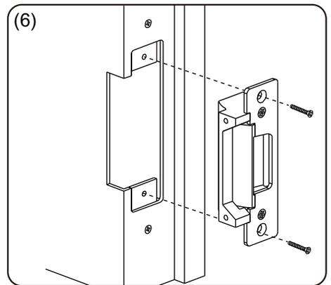
(6) Connect the wires, and install the strike
