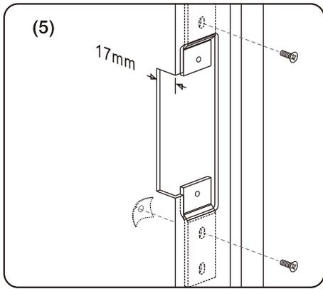
(5) Attach fixing lugs, and tabs if needed
